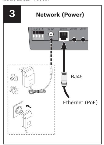
This equipment is only to be connected to PoE networks without routing to outside plant
